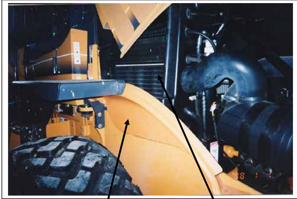
Removable fender well back in place.
