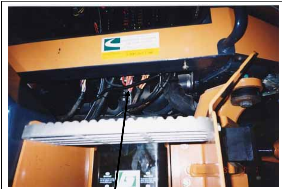
Clutch wire on right side of cab going up with hydraulic control lines
