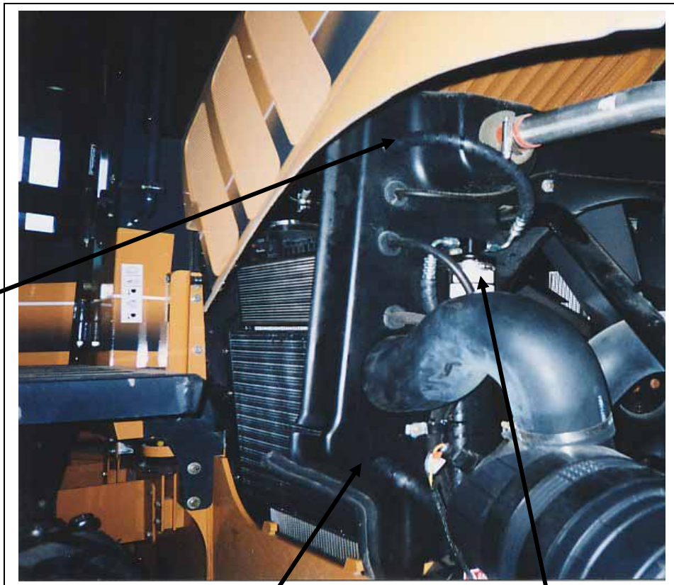
1 1/8" hole drilled in plastic shroud for 13/32" hose
