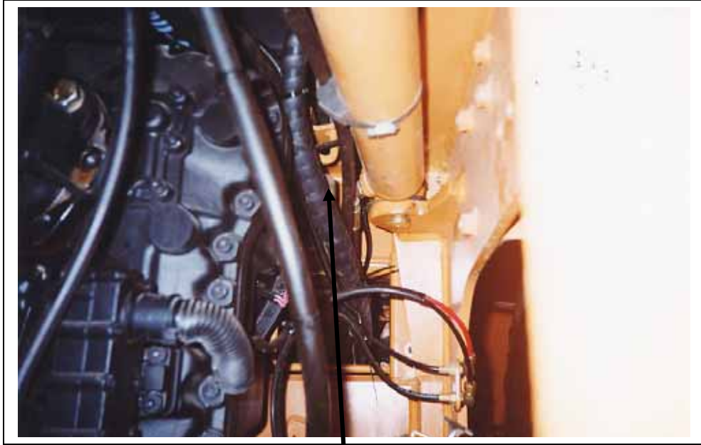
Hoses and clutch wire going back towards engine on left side of machine.
